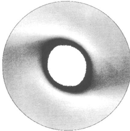
Fig. 2. The pair distribution function for the 32-particle soft-disk fluid at a relatively high reduced strain rate of 2.0. The reduced density and total energy per particle are 0.1 and 1.921, respectively. The run length is 24 million timesteps. The distribution is, as far as can be told from the simulation data, completely smooth. In spite of the high anisotropy of this distribution, the configurational contribution to the system entropy is only about 0.4%.
